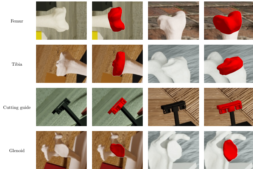
Figure 2: RGB images cropped around object of interest and respective estimated pose overlaid.
