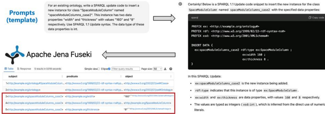
Figure 5: LLM for easier knowledge manipulation and query using GPT-4o
