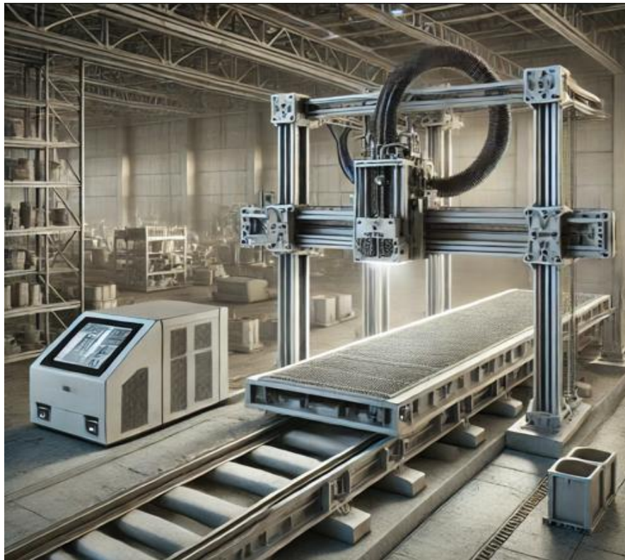
Figure 4. Gantry system of 3D concrete printer, created by AI
