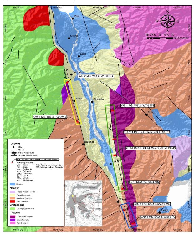
**Figure 1**. Geological map central part of Palu-Koro Fault zone showing sampling locality of the study area. The yellow line is the western segment, the green line is the eastern Segment and the blue line is the southern segment of the Koro Palu Fault, modified after [6].
