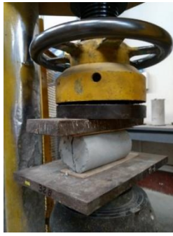
Fig. 2. Visualization of the failure in cylindrical concrete specimens by tensile test.
