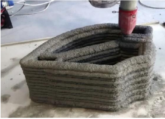
Figure 1: The printing processes (colour print) “Domenico Asprone et al. (2017)” [13]
