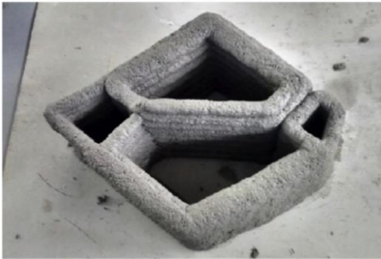
Figure 2: A printed Concrete segment (colour print) “Domenico Asprone et al. (2017)” [13]
