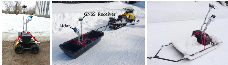
Fig. 5: Left : Rack mounted on a small robot for easy terrain (e.g. parking lot, sidewalks). Middle : Rack pulled by a snowmobile for maps on hardened snow. Right : As a last resort, the rack could be pulled by humans, which has proven to be useful on narrow/dense paths in the forest.
