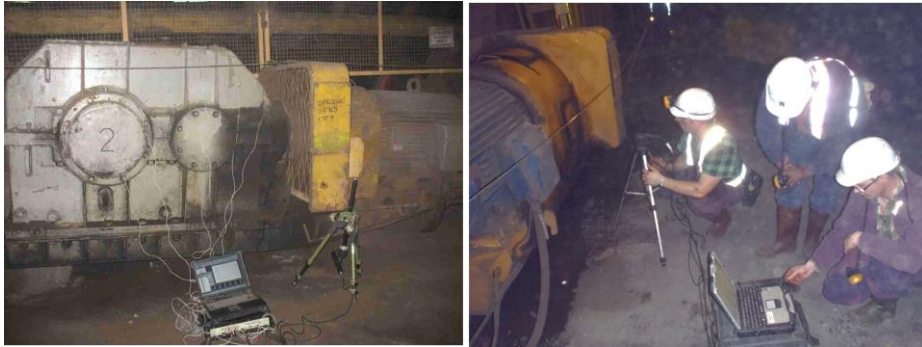
Fig. 5. Maintenance inspection for conveyor gearbox in underground mine - vibration measurement.
