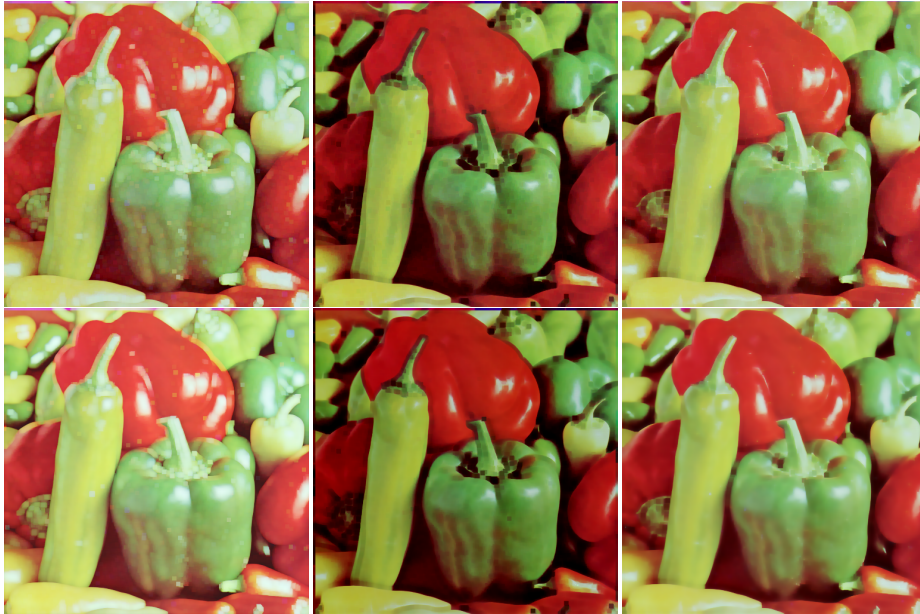
Fig. 1. Component-wise morphological operations with flat square 7 \times 7 filter on 512 \times 512 Pepper image. Top row: Classical method. Bottom row: Proposed fast approximations. From left to right: Dilation, erosion and closing.
