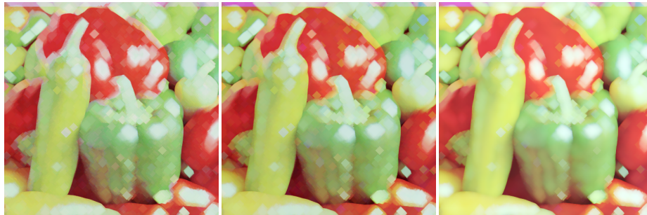
Fig. 4. Dilation of 512 \times 512 Pepper image by flat 21 \times 21 diamond shaped SE. Left: Loewner. Centre: Classic component-wise. Right: Proposed fast method
