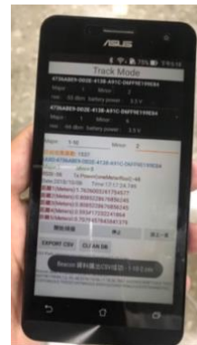
Fig. 11 The application of collecting RSSI signal
