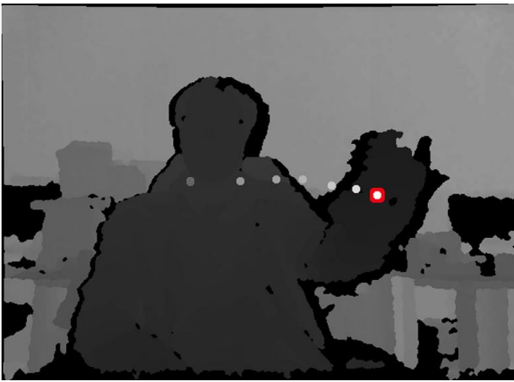
Fig. 8. Tracking of hand based on Kalman filter.
