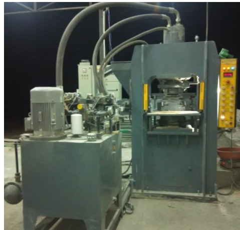
Fig. 4 Applying pressure on material by Hydraulic Compression Machine
