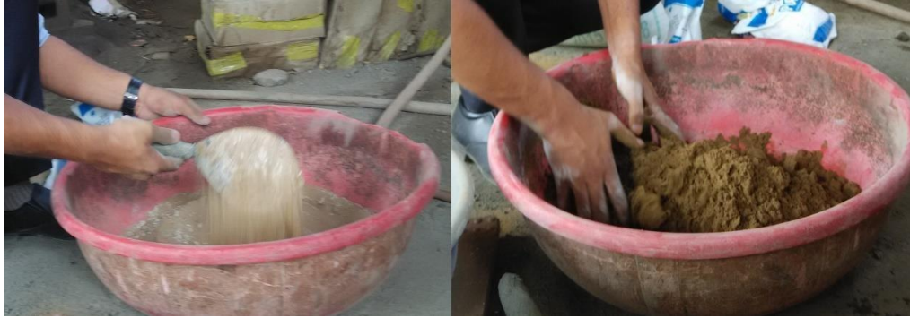
Fig. 3 a) Dry Mixing of all ingredients b) Wet mixing of all ingredients
