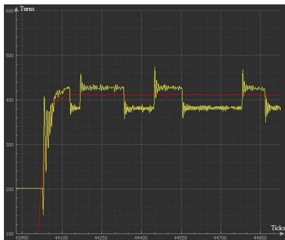
Fig. 13. Graph of the system behavior with PID-control
