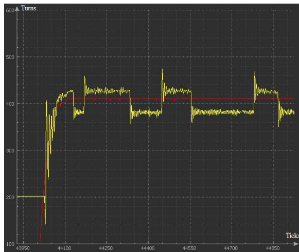
Fig. 12. The result of the PD-controller operation
