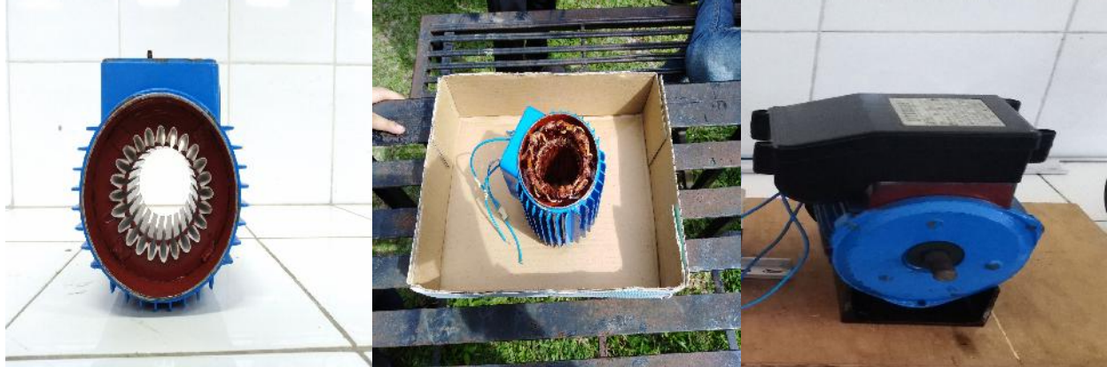
FIGURE 9. PSC motor with its new windings configuration after assembled
