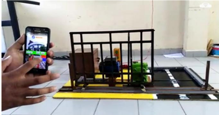
FIGURE 10. Sliding gate opener system together with the smartphone as its remote controller
