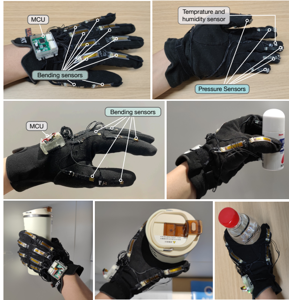
Figure 5: Our glove with bending (flex) sensors, pressure sensor, and temperature and humidity sensors.
