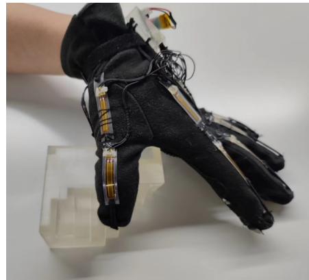
Figure 10: Bending Sensor Angle Testing Experiment Figure
