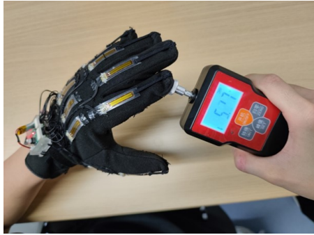
Figure 15: Pressure Sensor Testing.
