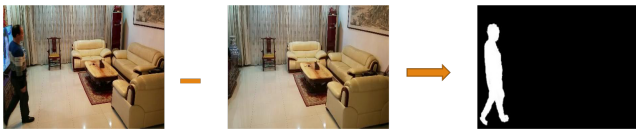
Fig. 2: Frame Difference Background Subtraction
