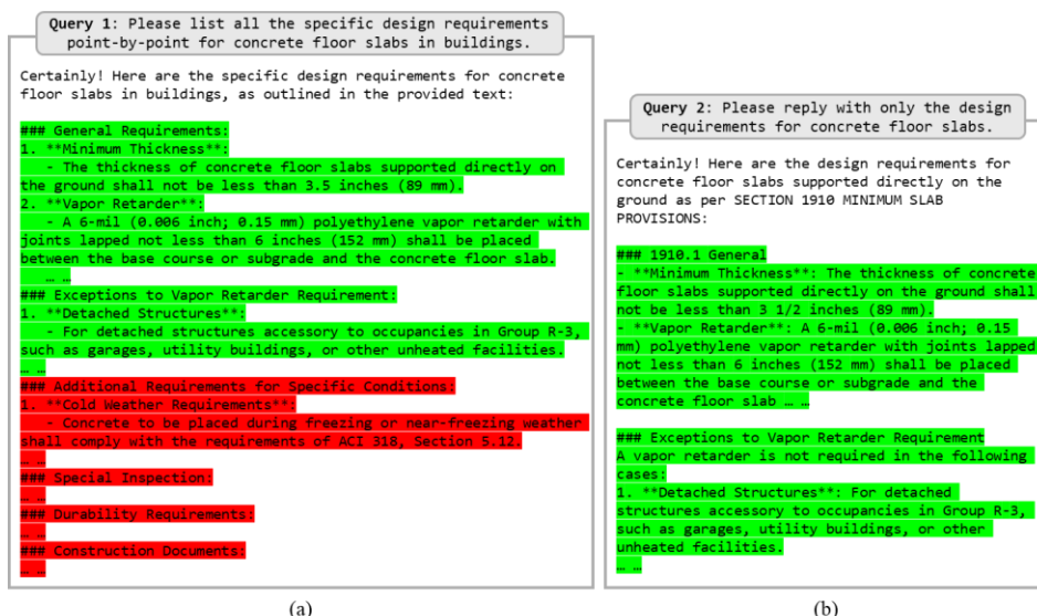
Figure 5. Two rounds of conversation for design requirement query: (a) first round; (b) second round. Note: the requirements colored in green are correct and those in red are irrelevant; "... .." indicates where text has been omitted for brevity.
