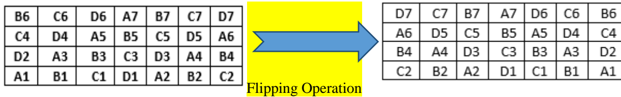
Fig. 6 b (flipping operation of the 7 bits)
