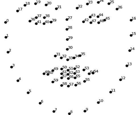
Fig. 1. Dlib model points for face detection with 68 points
