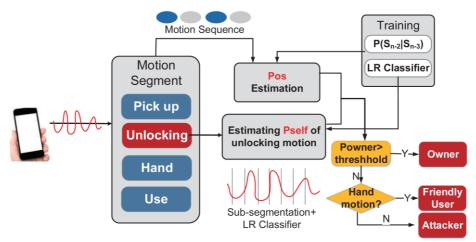
Fig. 3. Overview of MAS(Motion-sequence Authentication System)
