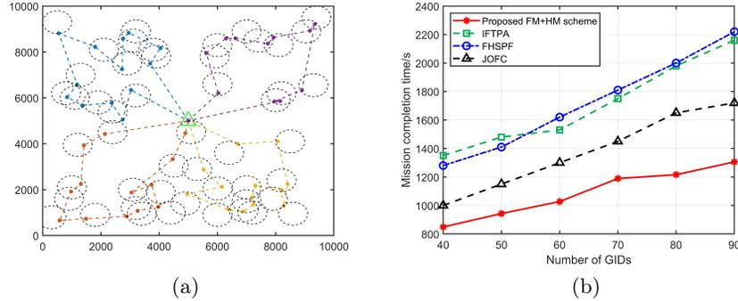
Fig. 2: (a): The final trajectory of the proposed scheme of combining FM with HM. (b): The mission completion time with diverse number of UAVs.
