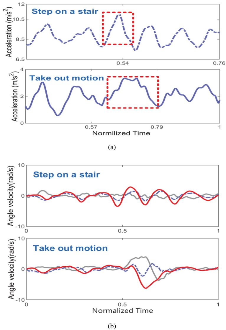
**Fig. 4.** The difference between take-out motion and step on a stair: (a) accelerometer data; (b) gyroscope data.
