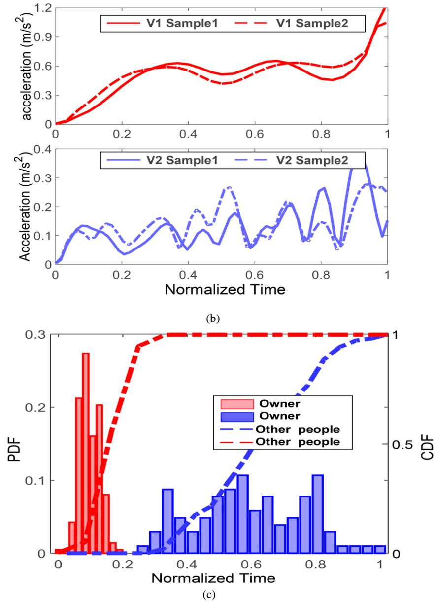
**Fig. 2.** The macro button chooses the correct format automatically. The unlocking motion performed by different people: (a) time series of velocity sampled during unlocking motion; (b) time series of acceleration sampled during unlocking motion; (c) distribution of normalized time distance between different users (e.g., owner and other people). PDF: Probability Density Function.
