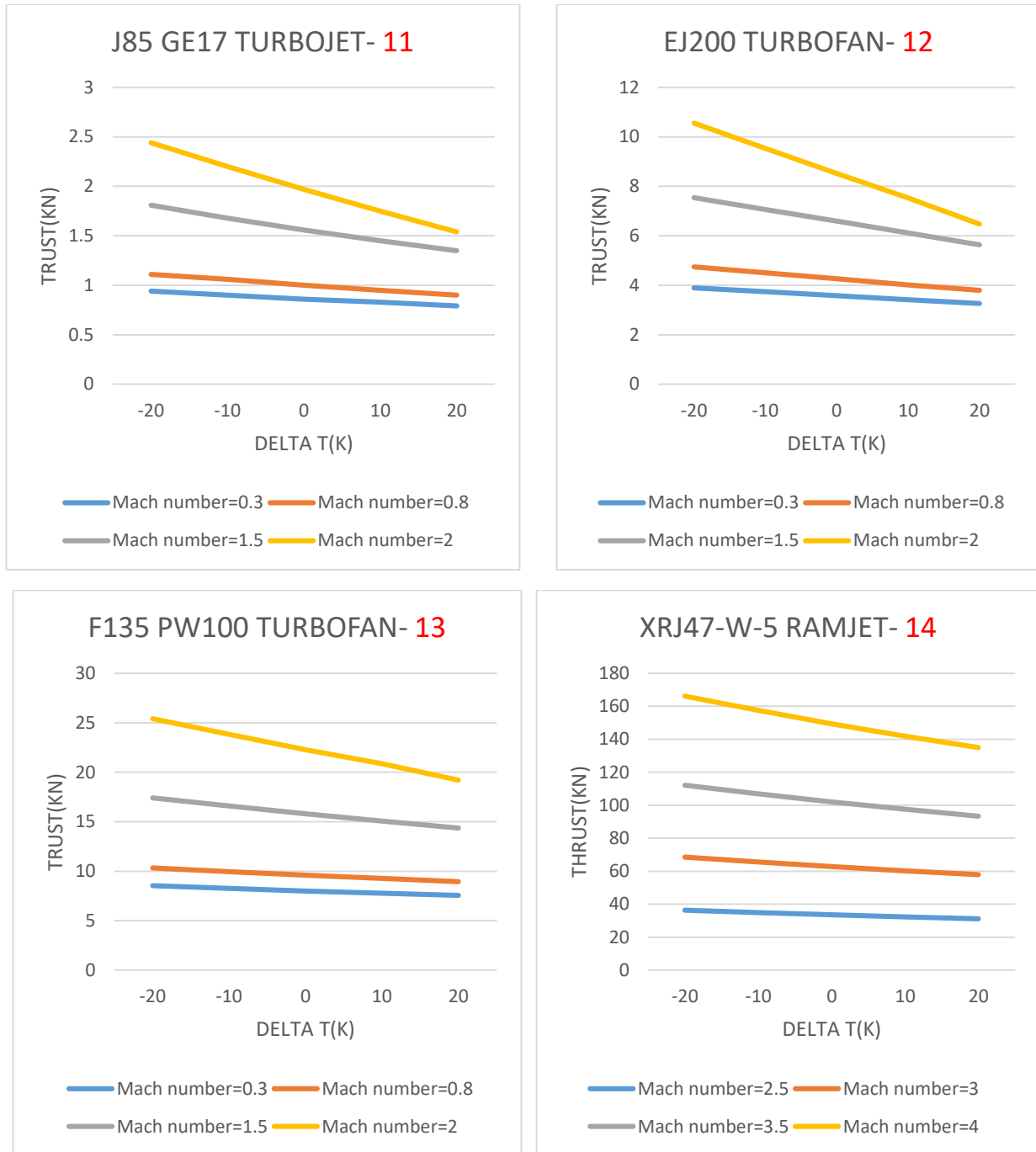
Figure 26: Thrust changes for J85GE17 turbojet, F135 PW100 turbofan, EJ200 turbofan, XRJ47-W-5 ramjet engines at an altitude of 20,000 meters and for hydrogen fuel with changes in inlet air temperature. Fuel flow rate changes for J85GE17 turbojet, F135 PW100 turbofan, EJ200 turbofan, XRJ47-W-5 ramjet engines at an altitude of 20,000 meters and for hydrogen fuel for J85GE17 turbojet, F135 PW100 turbofan, EJ200 turbofan, XRJ47-W-5 ramjet engines. It is shown in figure ( ) with the changes of the inlet air temperature. Since the actual flow rate of the inlet air increases with the decrease of the inlet air temperature, more thermal energy is needed to
