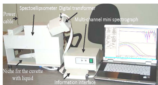
Fig. 11. Adaptive Identifier (version 3) based on the 35-channel spectroellipsometer
