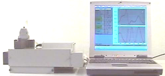
Fig. 9. Adaptive Identifier (version 1) based on the 128-channel spectroellipsometer and oriented to the laboratory analysis of liquid samples.
